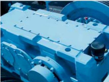
Automated rail mounted gantry crane (ARMG) with bevel-helical gear units and brakes
